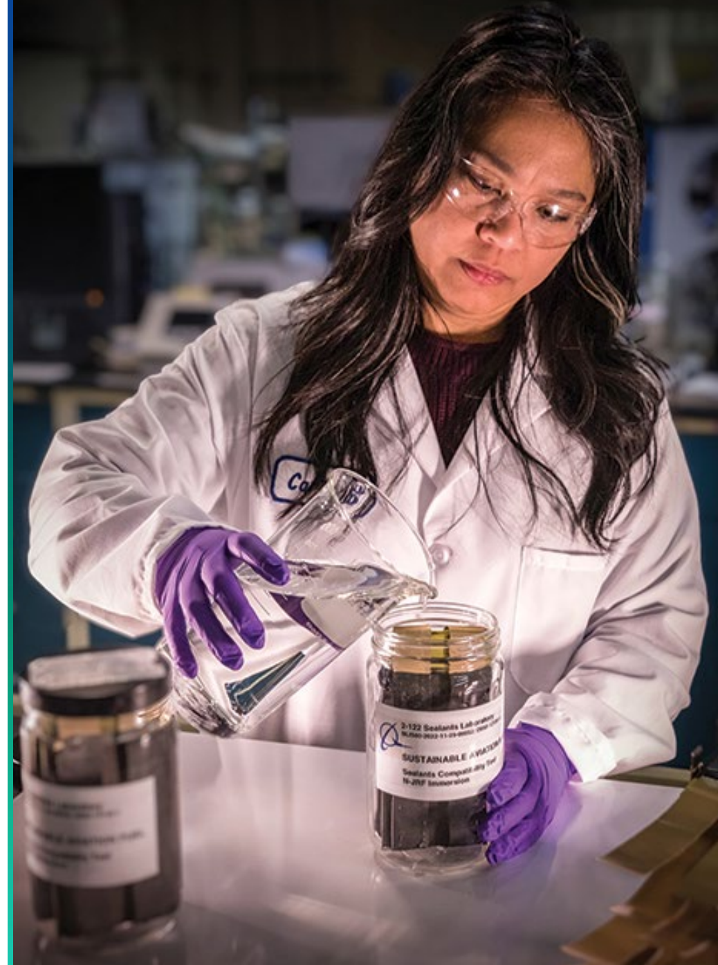
Boeing engineer pours jet reference fluid into a jar for sealants immersion testing in a laboratory.
